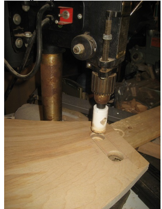
Drilling Finger Cutouts
